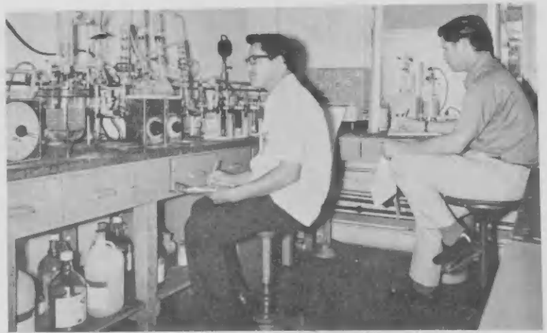
Lab Assistant Virgilio Angela (left) determines nitrogen in HDS components with Kjeldahl distillation apparatus. At right, Lab Assistant Alberto Penja makes analysis of catacarb and MEA solutions using the automatic titrometer.
